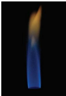
Figure 16. The tip of the inner blue cone is the hottest part of a flame. © Erin Taylor
