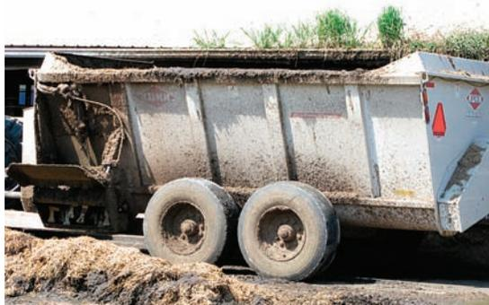
Figure 15. Slinger spreader used for spreading manure and compost. © Erin Taylor
