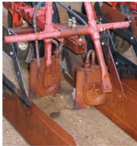
**Figure 6. Burners need to be staggered to avoid turbulence, which makes flaming less effective.** © Erin Taylor
