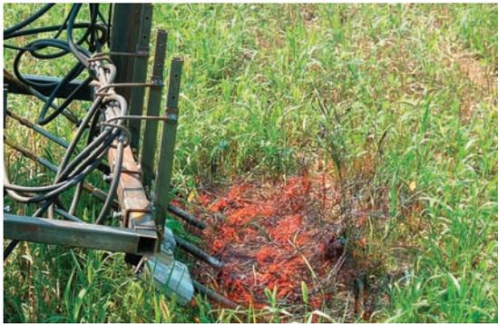
Figure 2. Broadcast flamer with four burner units set 12 inches apart. © Stevan Knezevic
