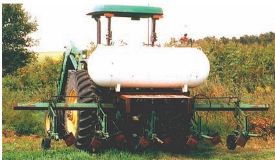
Figure 1b. Three point hitch mounted 4-row flamer with 2 burners per row set perpendicular to the row at a ~60 degree angle to the ground. © Ron Dunphy
