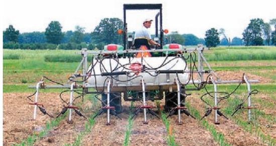
Figure 3. Flaming at the base of corn plants controls weeds within the row. © Erin Taylor
