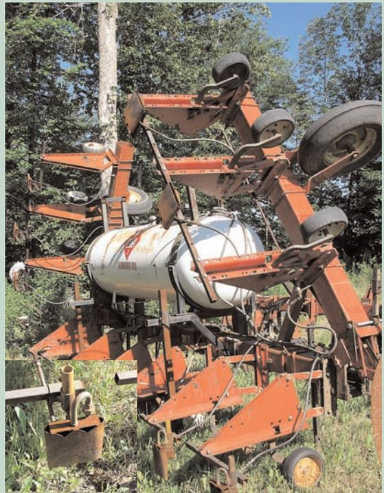
Figure 22. Three point hitch mounted 12-row flamer with one burner aimed directly over the row (lower left) built by Gene Vogel. © Erin Taylor
