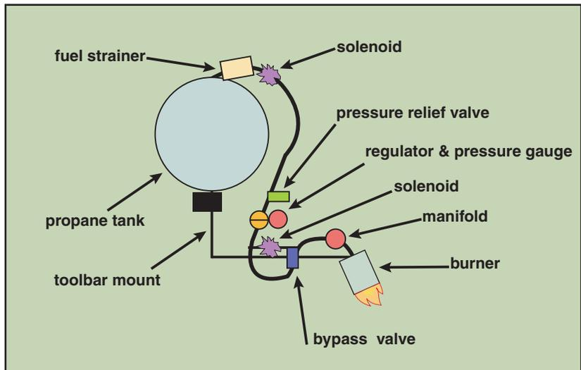
Figure 5. Basic components of a band flamer.
