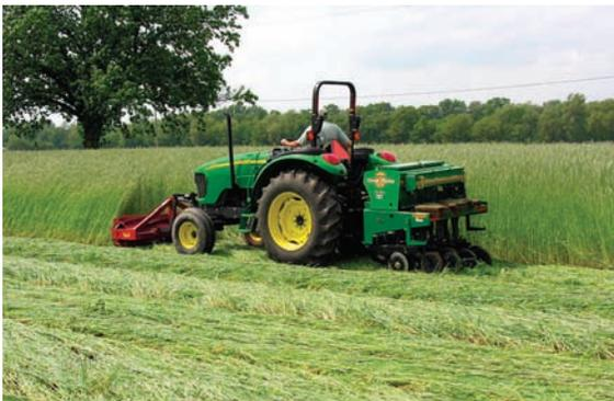
Figure 27. Crimping rye and planting soybeans in one pass Kellogg Biological Station. 📷 Todd Martin
