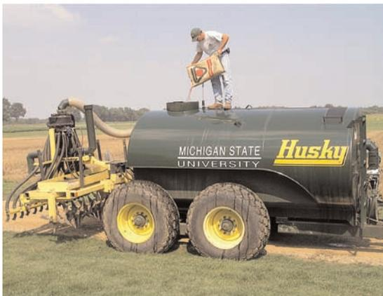
**Figure 21.** Cover crop seed is added directly to the manure slurry in the slurry tank. Bypass flow from the pto-driven pump provides seed agitation and mixing. © Tim Harrigan
