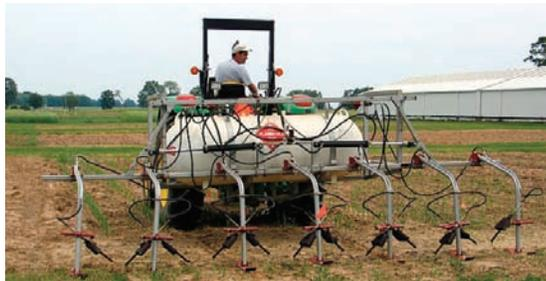
Figure 1c. Three point hitch mounted 6-row flamer with 2 burners per row, set perpendicular to the row at a 45° angle to the ground. © Erin Taylor
