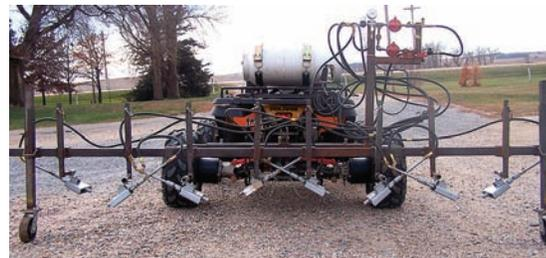
Figure 1d. Four-row research flamer with 2 burners per row set perpendicular to the row at adjustable angles. © Stevan Knezevic
