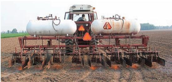
Figure 1a. Pull behind 8-row flamer with 2 burners per row directly over the row. © Erin Taylor
